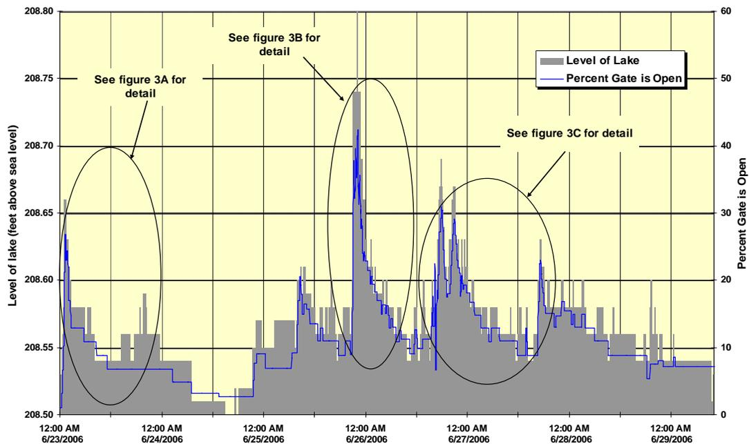
Lake level is compared to the percent of gate opening in Chart 3 to illustrate how closely the gate opening is linked to changes in water level. The left scale, corresponding to lake level and represented by the solid grey areas of the chart, is contrasted with the percent of gate opening, shown on the right scale and represented by the thin (blue, if color) line.
