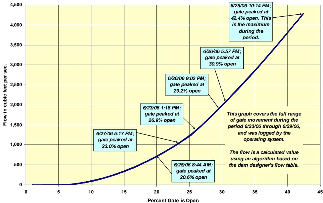
Notice in Chart 1, which relates the percent of gate opening (bottom scale) to the flow over the dam (right scale), how the first 10% passes only a minor amount of water. As the gate opens wider, flow increases less than proportionately with only about 20% of flow capacity passing over the dam at 40% of gate opening. Only above 40% does the flow increase become roughly linear.
